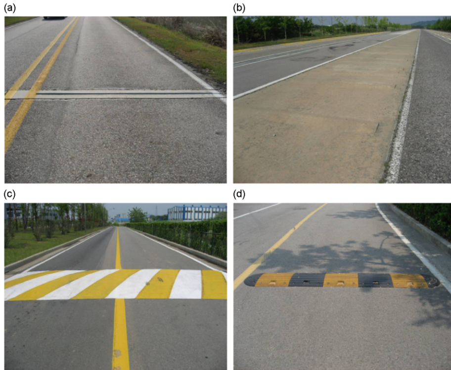
Fig. 3. Photographs of the test courses. (a) Course 1: impact bar, (b) course 2: continuous bandy road, (c) course 3: broad bump, (d) course 4: narrow bump.
